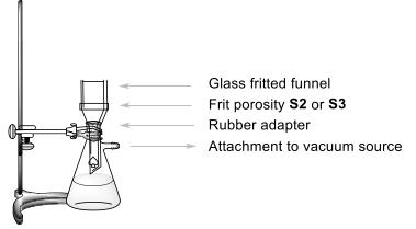
Figure 3. Setup for suction filtration.
