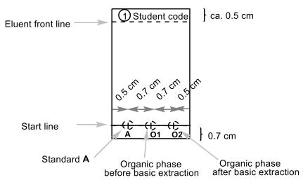
Figure 2. Instructions for the TLC plate preparation.
