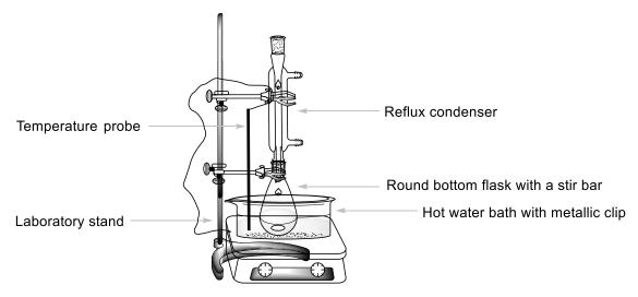
Figure 1. Setup for heating the reaction mixture in a water bath.
