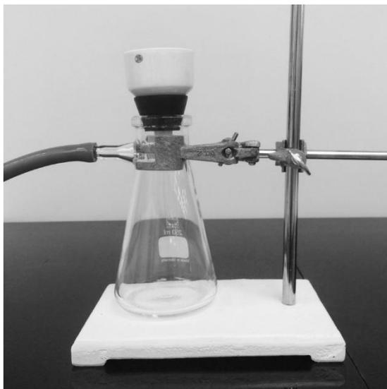
**Figure 2:** Set up needed for suction filtration.
